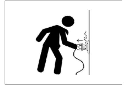
15. If you detect an increase of temperature in an appliance during operation, disconnect it immediately from the mains, investigate the reason and repair it before reconnecting.
